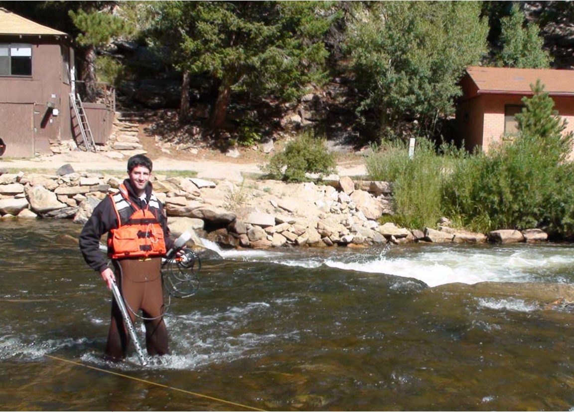
Carefully measuring the discharge rate every three feet, across the Big Thompson River.
